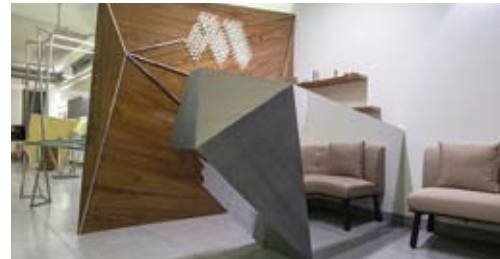
Reception desk in satin, mirror polish and gunmetal finish SS, with veneered partition backdrop featuring firm logo signage in backlit acrylic rods.
