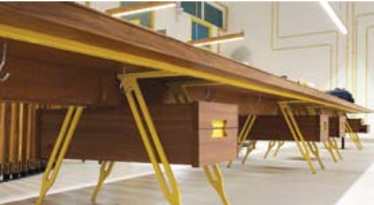
The detail of the main central workstation shows MS framing and waterjet cut legs, with drawer boxes and bag hooks slung below the worktop.
